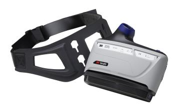
The 3M™ Versaflo™ Powered Air Turbo TR-600 is a belt-mounted air purifying device. It can be combined with an approved headtop or facepiece to form a power-assisted system for respiratory protection against particles, nuisance odours (where applicable) and gases and vapours. A range of approved breathing tubes are available depending on which headtop or facepiece is selected.
