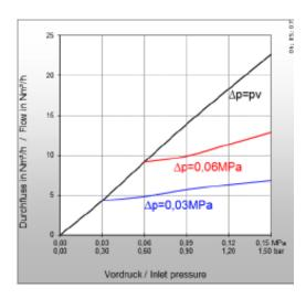
\* Conversion factor 2.5 for devices comprising a flame arrestor The conversion factor for free flow is 3.8 ( Reference: BAM report 220, D .Lietze)
