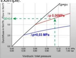
QG = QD x F QG  $\blacktriangleright$  A = 6,4 x 1,2 = 7,68 m<sup>3</sup>/h C2H2 QG = flow / gas type F = conversion factor QD = flow / air
