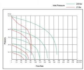
"FLOW TAKEN UNDER STANDARD WORKING TEMPERATURE OF 25"C +-1.5"C USING OIL FREE BREATHABLE COMPRESSEDAIR, WITH DIGITAL FLOW DEVICE (SERIAL NO.00763)CALIBRATED TO FULL SCALE PRESSURE 160PSW WITH AN ACCURACY OF +1-0.5% OF FULL SCALE PRESSURE.
